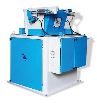
Net weigher pre-weighs the material in weigh hopper & discharges it into bag. Systems is available with single & dual weigher option for weigh range from 5 to 100 kg per weighment.
